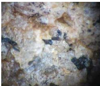
8x magnification after cleaning with ROTEC VORTEX cleaning system no etching visible. Photo courtesy of JMC Stone Co.
